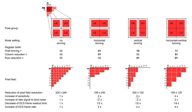
Figure 41: Pixel binning modes and readout
