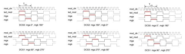
Figure 49: 4 DCS modulation/demodulation waveforms
