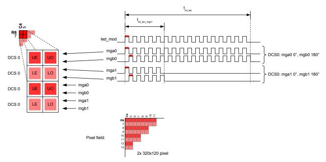
Figure 40: Dual integration time mode: even and odd rows independently controlled by mgx0 and mgx1. One stops earlier than the other.
