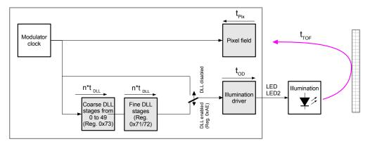
Figure 22: Block diagram of the DLL function
