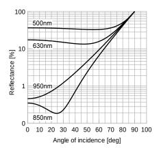
Figure 4: Reflectance vs. illumination angle (AOI)
