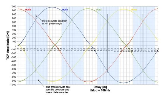
Figure 23: DCS amplitudes for the 4 DCSx (measurement data)
