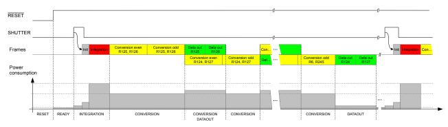
Figure 55: Power consumption levels and operating states
