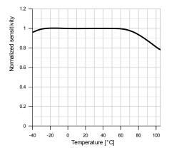
Figure 7: Typical TOF sensitivity temperature coefficient
