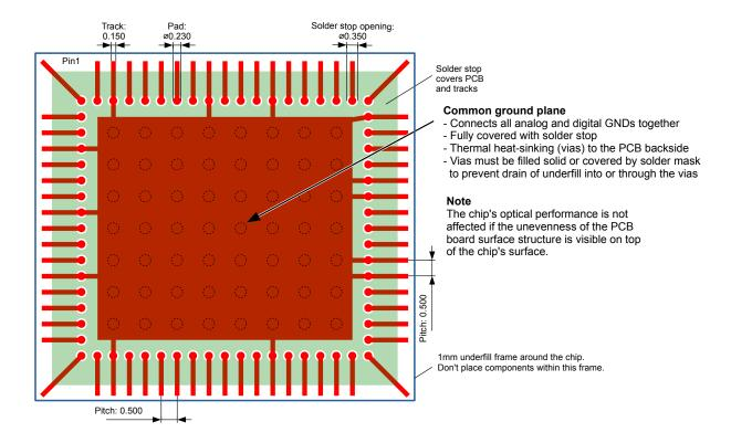
Figure 13: Recommended PCB layout (all measures in mm)
