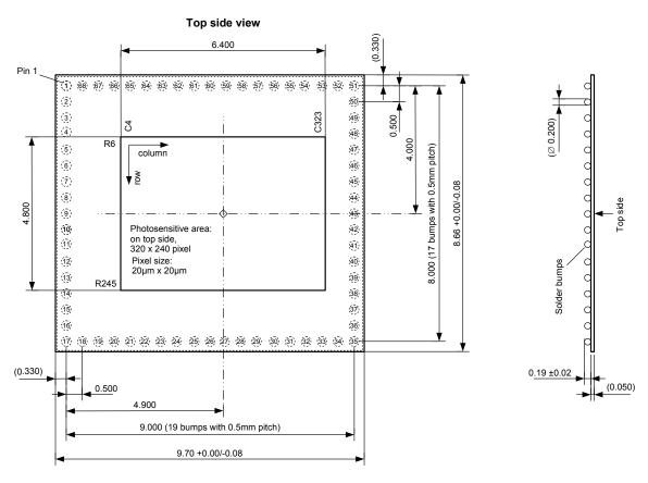
Figure 10: Mechanical dimensions
