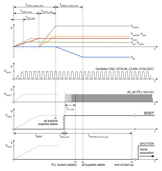
Figure 21: Power-up and reset sequence
