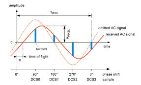
Figure 52: Sampling of the received waveform
