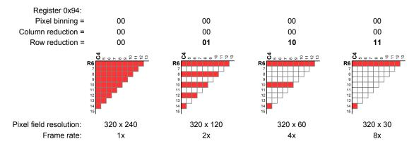
Figure 42: Row reduction on y-axis without binning
