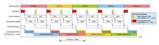
Figure 57: Enhanced rolling mode sequence
