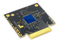
Figure 16: epc660 CC Chip Carrier, refer to separate datasheet
