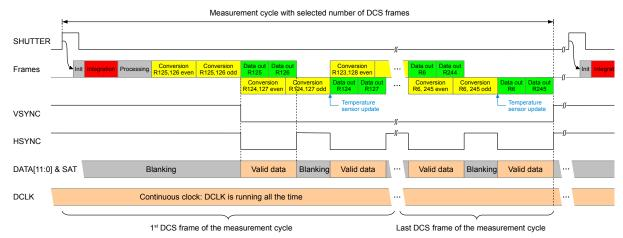
Figure 26: Continuous clock mode
