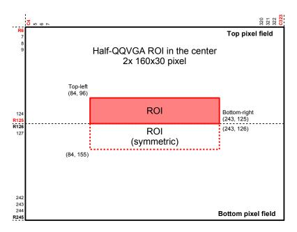
Figure 35: ROI for Half-QQVGA: 2 x 160 x 30 pixel
