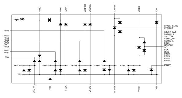
Figure 9: I/O pins and ESD protection diagram
