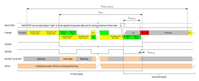
Figure 30: Frame timing: Inter frame timing, end of frame and start next frame
