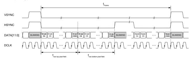
Figure 31: 12-bit mode data readout
