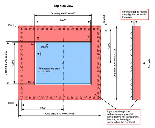
Figure 11: Opaque cover for protection against unwanted ambient-light
