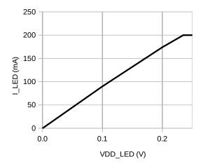
Figure 18: Output characteristic  $I_{\text{LED}}$  versus  $V_{\text{DDLED}}$ . Refer for maximum values of  $V_{\text{DDLED}}$  and  $I_{\text{LED}}$  to Table 1 and Table 2
