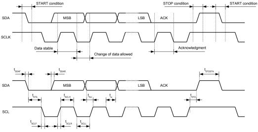
Figure 60: I2C bus timing
