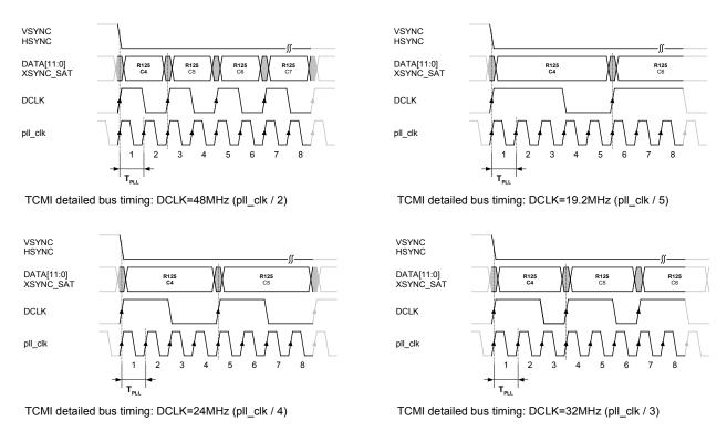
Figure 28: TCMI timing examples with symmetric and asymmetric DCLK
