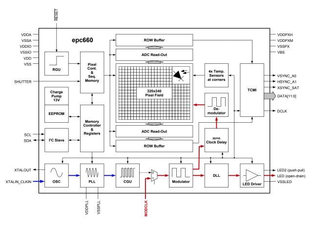
Figure 20: The MODCLK signal flow (red marked)
