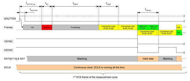
Figure 29: Frame timing: Start 1st DCS frame
