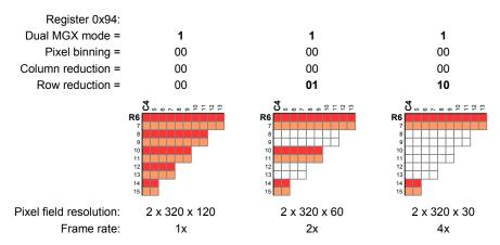
Figure 46: Row reduction on y-axis combined dual phase mode
