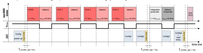
Figure 54: Sequence for normal DCS mode
