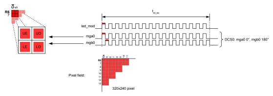
Figure 38: Full resolution mode: even and odd pixel rows are controlled identically with mgx0
