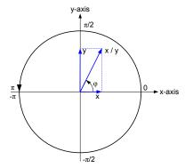
Figure 51: Continuous atan2 representation for the range  $-\pi$  ...  $+\pi$
