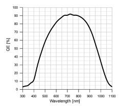
Figure 6: Typical quantum efficiency
