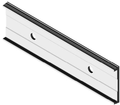
2.) Fix the mounting plate with two screws with a maximal screw head height of 2.8mm. (e.g. M3 cross-head screws, M3 hexalobular screws or ST3.5 tapping screws etc.)
