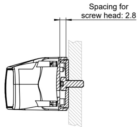
3.) Clip the camera onto the mounting plate
