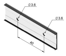
2.) Fix the mounting plate with two screws with a maximal screw head heigt of 2.8mm. (e.g. M3 cross-head screws, M3 hexalobular screws or ST3.5 tapping screws etc.)
