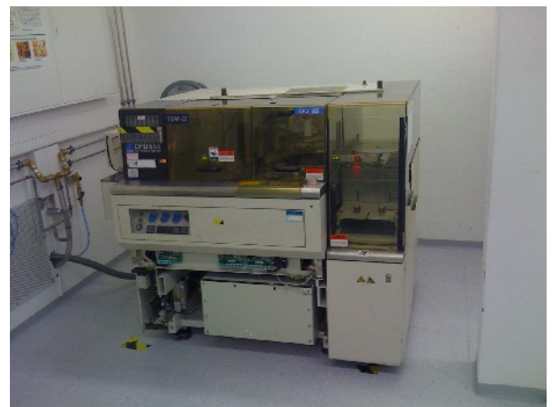
New dicing machine in our cleanroom in Sargans
