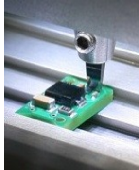
Shear test to qualify bonding joints
