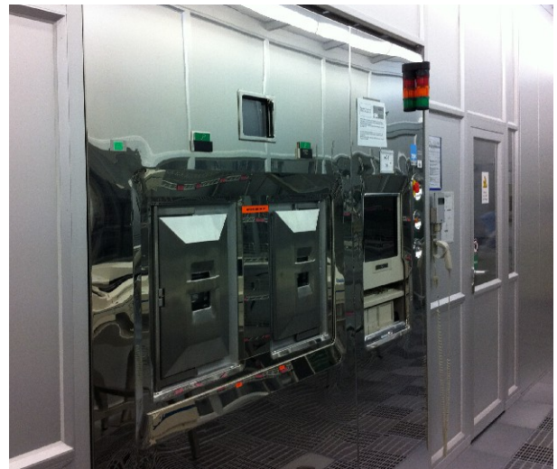
An implanter, such as the one pictured here, will be installed in the second cleanroom during 2012.
