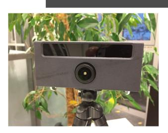
At Photonics West we will show an FPGA-based QVGA TOF camera in an open-frame design (the picture shows the camera in a housing). This camera is designed to be implemented into applications like automated guided vehicles (AGV) or any other mobile robot which requires 3D ambient infor-
