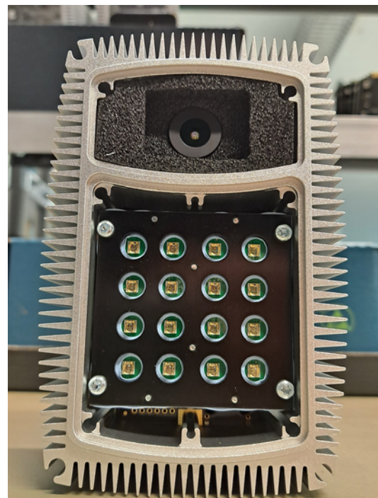
TOFcam-660 in production. Application for the customer: Fall detection
